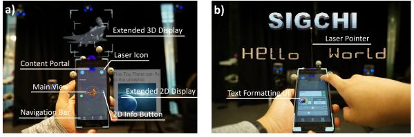
\*Figure 1. We explore joint interactions between an Augmented Reality Head-Mounted Display and a smartphone. a) The HMD can be used to enhance smartphone interactions, for example, by displaying in-place previews of 3D content. b) The smartphone can be used to enhance AR centric task, for example, by supporting object selection or detailed UI configurations.
