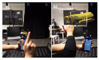
Figure 6. A freehand air tap and drag gesture can be used to move augmented content in the environment.
