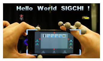
Figure 12. In Group Select mode, a swipe along the top of the phone performs a top alignment of the selected objects.
