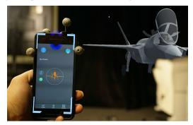
Figure 9. A full screen rotation widget can be used to make small adjustments to the model's orientation.
